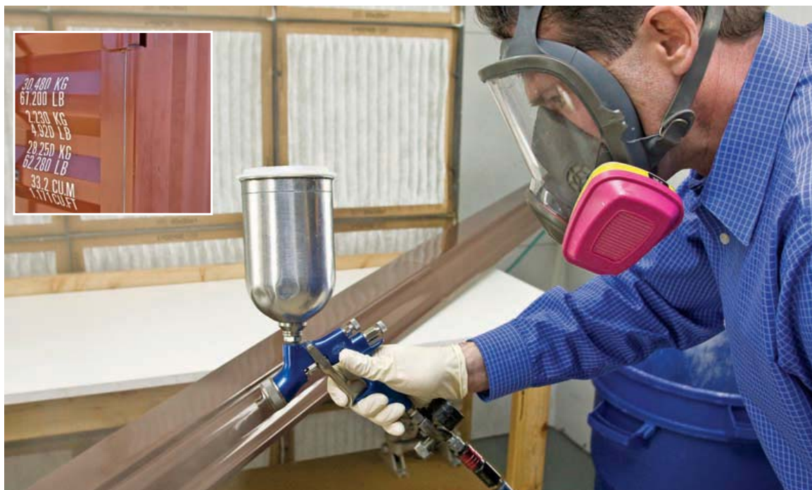
[PHOTOS BY CARTER SHERLINE] Nanovere Technologies founder Tom Choate (above) sprays a layer of Nano-Clear, which he says preserves surface gloss and resists scratches and oxidation. Compare the side on the left without coating to the side on the right with it (inset, above).
